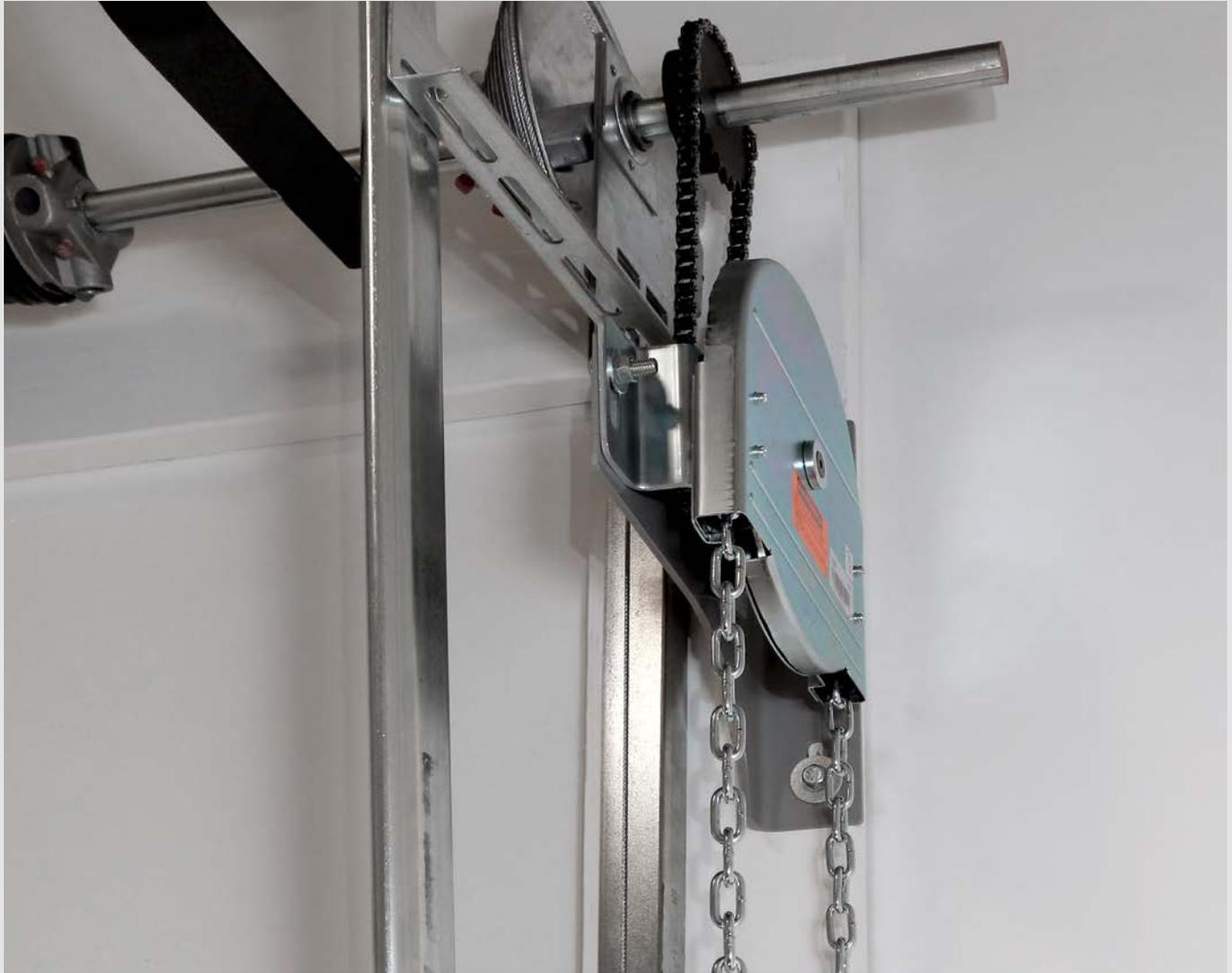
The Safe-T-Stop™ chain hoist features an integral braking system that allows the door to move only when the user is actively pulling the chain. Unlike standard chain hoists that can allow the door to move out of control, this hoist allows users to operate the door more safely. The Safe-T-Stop™ chain hoist can be installed on new or retrofit applications and is ideal for vehicle service stations, restaurants, warehouses and drive-through doors.
